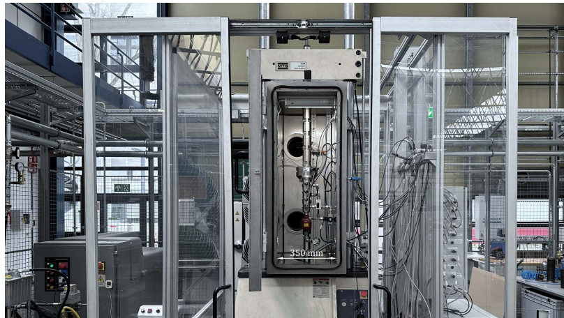
Figure 2: Uni-axial servo hydraulic test rig MTS 850 test damper at the chair of Fluid Systems at Technische Universität Darmstadt
